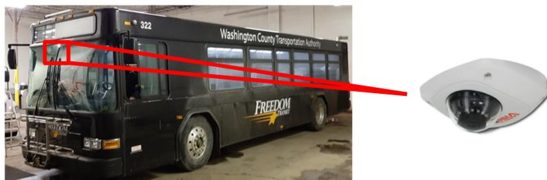
The bus is equipped with 5 cameras, 4 of which are mounted on the outside of the bus. We use the dash cam which is mounted inside to avoid foggy images that may appear in wintry weather.
